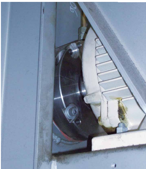
Espey WDKS-Eco, installed on a kiln housing Photo by courtesy of Aurubis AG
