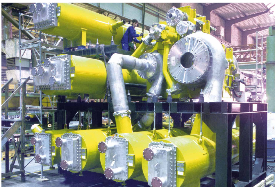
Multi-stage gear compressor Photo: MAN Diesel & Turbo SE
